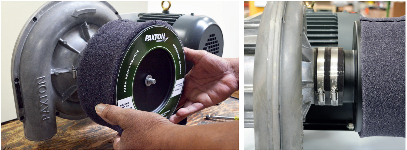
18. Reinstall filter and housing.
